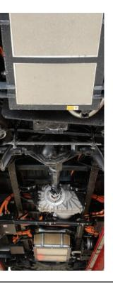
the batteries (three) plus the onboard charger.
